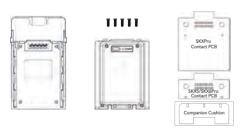
2. Remove the transparent protective tape from the back of the companion cushion and attach it to the back of the SKXPro as shown below. (C)
