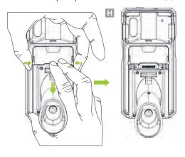
3. Close the battery door and turn the battery door knob clockwise to lock. (K)
