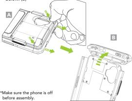
2. Slide the XCover smartphone into the SKX SmartSled and flip the top cover forward as shown. (C)
